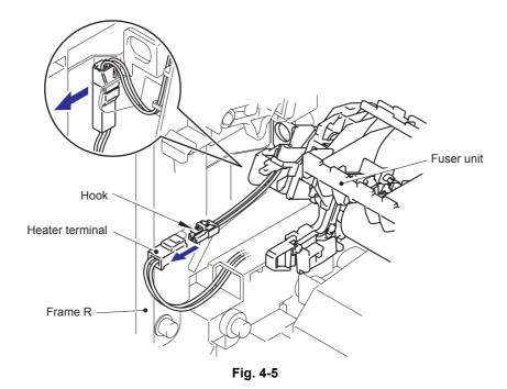
(10) Pull the FU harness cover 2 to the direction of 10a while pressing the Hook and pull out the FU harness cover 2 from the back of the printer.
