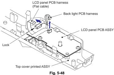
(3) Remove the three cup B M3x8 Taptite screws, and then remove the LCD panel PCB ASSY.
